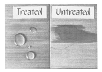
For example, in tests conducted near Madison, Wisconsin, a water-repellent solution containing paraffin wax and a small amount of drying oil or resin, but no preservative, protected window units from decay for 20 years. In these tests, paint weathered away after 10-12 years of exposure to the elements, but the wood remained sound. One caution: water-repellent treatments that lack a preservative may not prevent mold growth, especially in warm climates.
