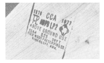
Treated wood marked "for above ground use only" should not be used in the ground. Use these materials only above ground — they contain less preservative than do posts treated for ground contact.
