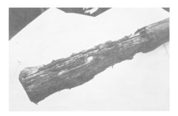
How long naturally decay-resistant wood lasts depends on the type of wood and the climate. Untreated, square, California redwood posts should last 4 to 20 years, depending on climate.
